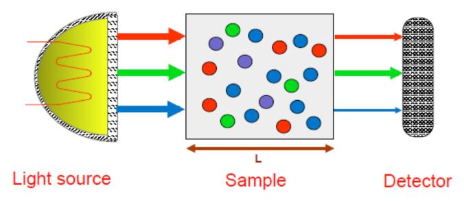
Length of optical path (L) affects measurement sensitivity
